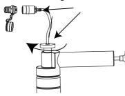
6. Thread probe to valve. Pull back on the handle to draw the purge sample. Purge volumes vary according to
