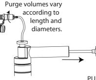
7. Unthread the probe, 2 turns only. This will close the valve.
