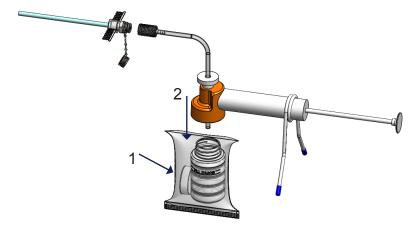
2) Keep the sample clean on a windy day by threading a zip bagged bottle onto the pump
