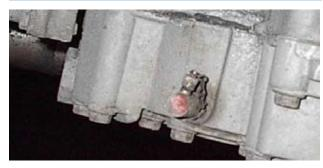
The most common install location for transmissions is the main pressure port. If the port is not directly accessible we will recommend a remote access solution which uses a hose assembly to extend from the port to a location it can be mounted. **Contact Checkfluid for more information on remote access solutions.**
